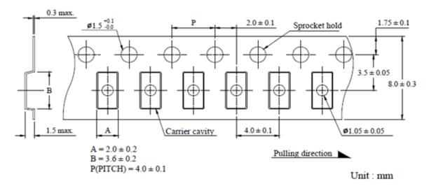
Remark: Leader tape length  $\geq$  30 cm( 150 Hollow carrier cavity)
