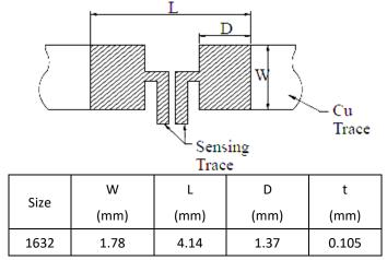
t: Copper foil minimum thickness of PCB
